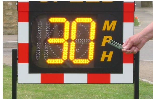
Easy calibration with 30MPH tuning fork
