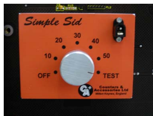
Simple SID's rotary switch operation
