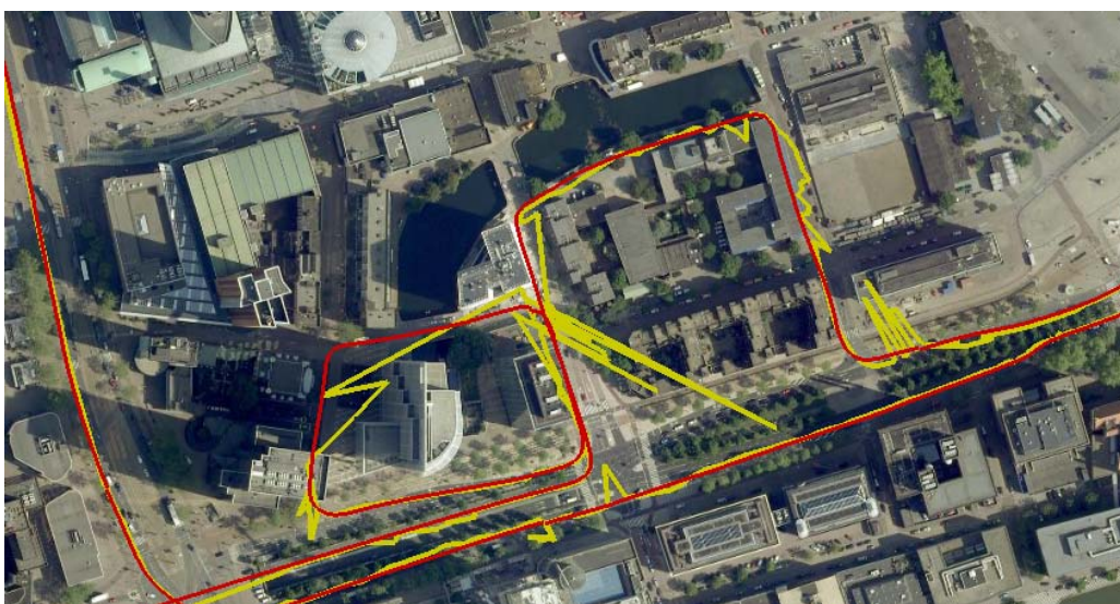
Plots of GPS-only (yellow) and Inertial+ (red) in an Urban Environment
