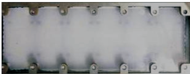
Figure 7: spreading behavior after tighten up the screws
